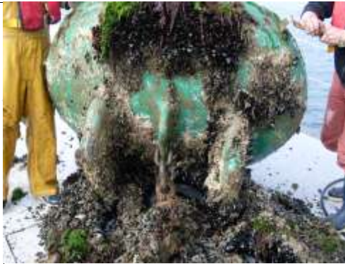
Figure 16 Removal of marine growth by scraping
