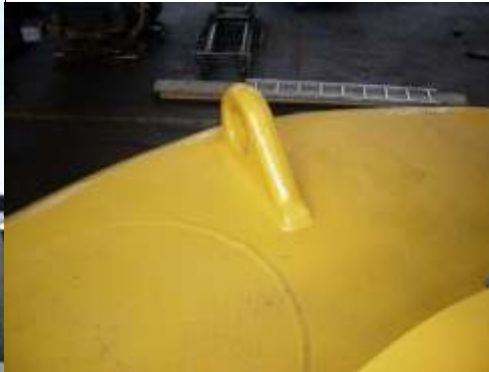
Figure 18 Check the lifting eyes
