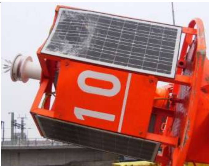
Figure 24 Damaged solar panel
