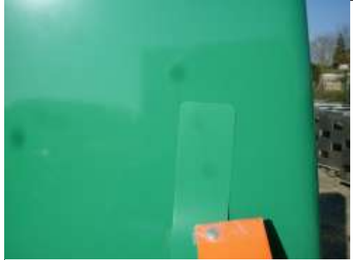
Figure 12 Confirmation of colour using reference card
