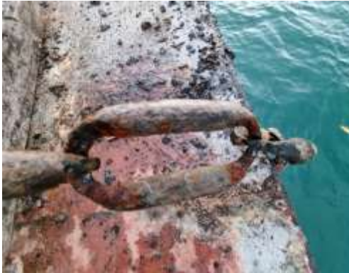
Figure 1 Chain Wear
