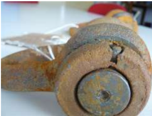
Figure 3 Example of excessive wear around shackle pin
