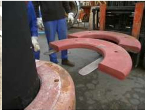
Figure 23 Replacement of ballast sections
