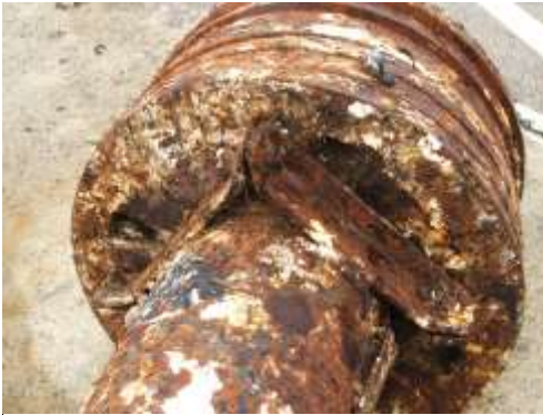
Figure 22 Heavily corroded ballast
