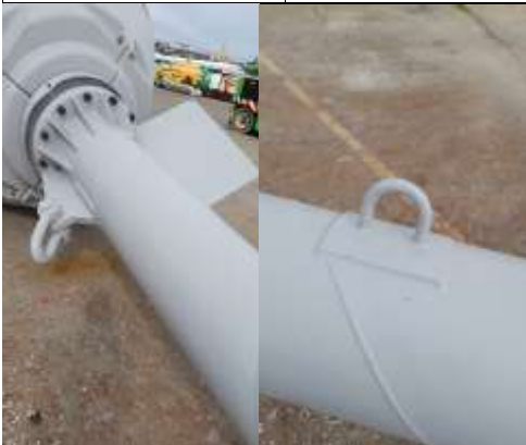
Figure 20 Check the drift plate and lifting eye
