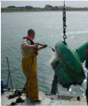
Figure 15 High pressure water jet cleaning of buoy
