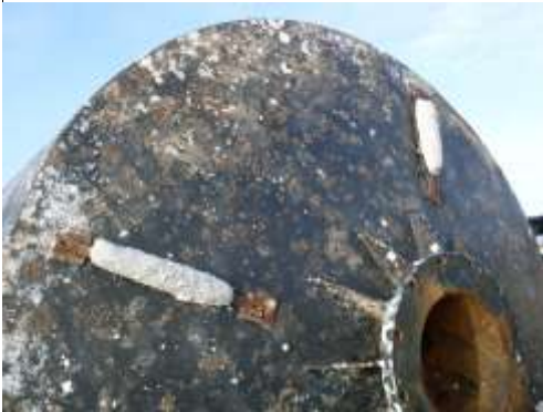
Figure 17 Check the sacrificial anodes
