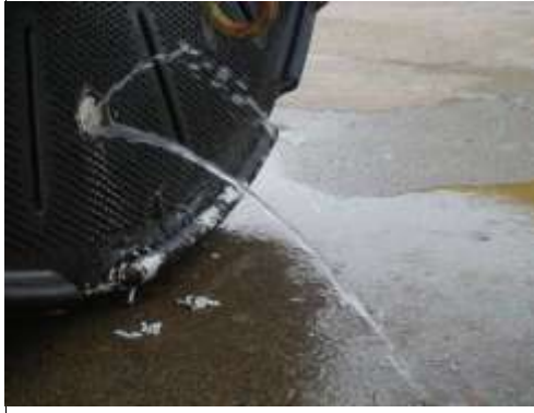
Figure 14 Water ingress in buoy floats may occur
